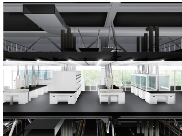
Installing an ISS above the experiment labs allows for reaction to change in research during operation
