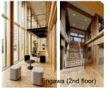
The Engawa is reinterpreted as a space that performs modern functions, such as using natural energy and natural ventilation to address global warming and climate change, and to reduce environmental impact. A vaulted porch around the perimeter of the office reduces the heat load in the rooms and contributes to more active staff communication as a comfortable space with natural ventilation. The workspace is designed to accommodate "activity-based working".
